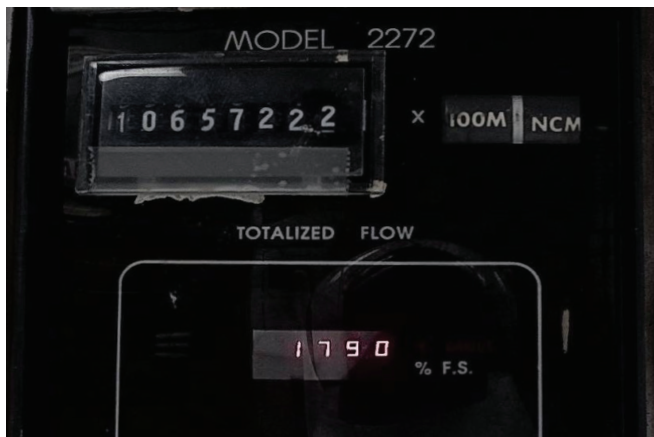
A camera is positioned facing the analog gauge, providing a continuous feed to the AgoraGateway running a machine learning algorithm to digitize the data in real time.
