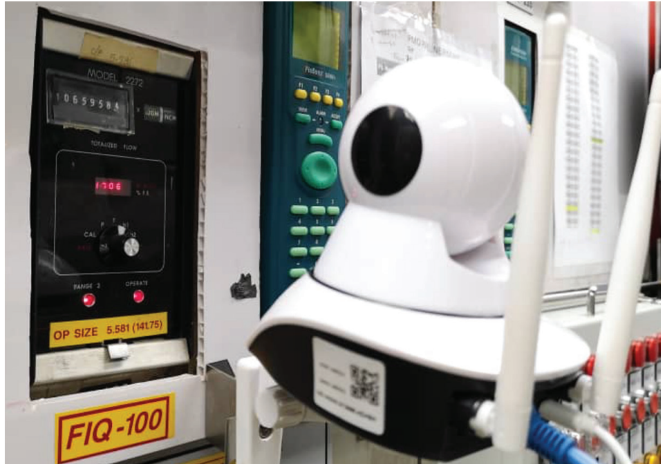
A camera is positioned facing the analog gauge, providing a continuous feed to the AgoraGateway running a machine learning algorithm to digitize the data in real time.
